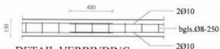
DETAIL VERBINDING OVERLAPPING WAPENING RINGBALK 150MM
